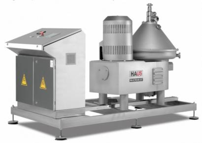
**THE PRODUCT** MAXCREAM 20T is a centrifugal separator configured as a concentrator for dairy application, with double paring discs, partial and total automatic discharge capabilities, and ready for Clean-In-Place (CIP).
